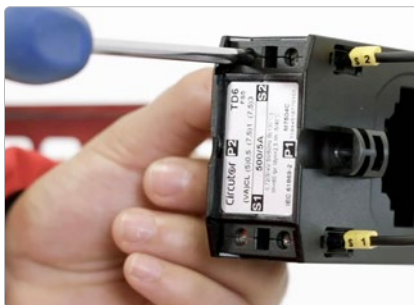
Connect the secondary cables.
