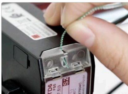
Once the terminal cover has been placed, the transformer sealed.
